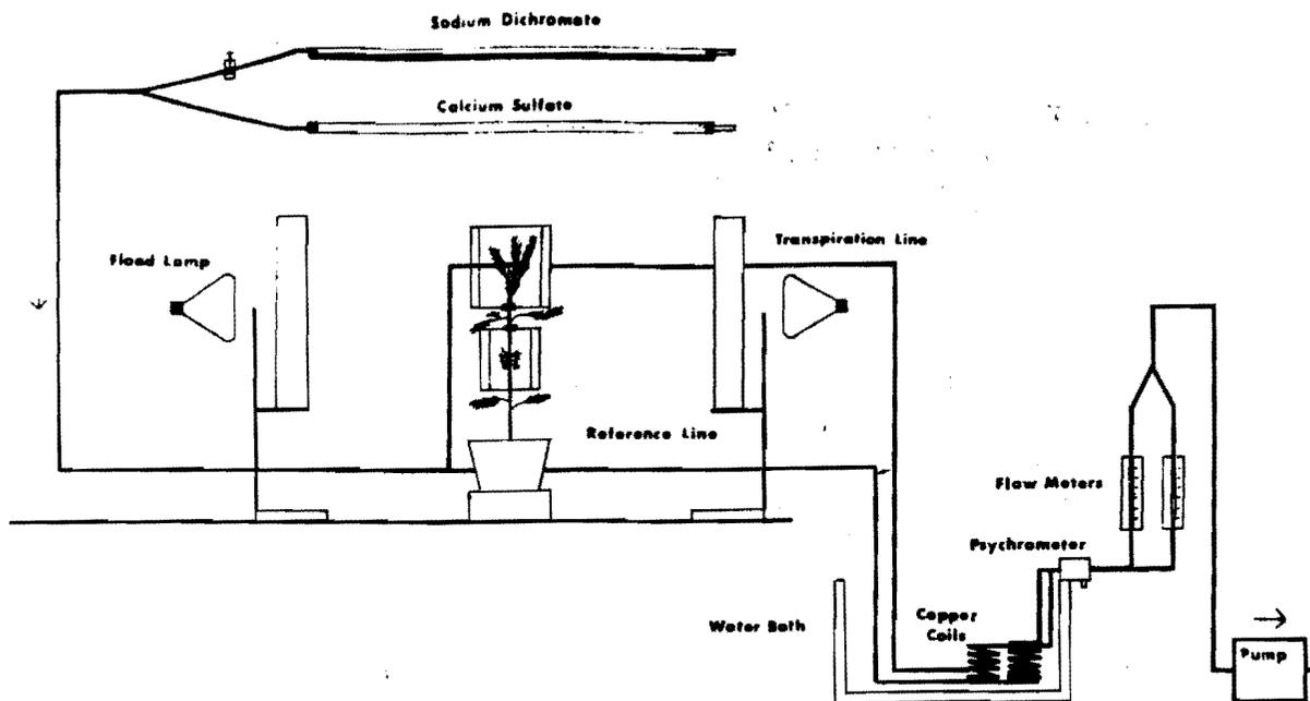
Figure 1. Schematic representation of apparatus used to determine transpiration of A. americanum and lodgepole pine.
