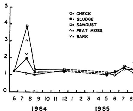
Figure 1.--Effect of organic amendments on soil test OM at the Albuquerque Tree Nursery. Only the peat moss treatment is significantly different from the control ( $\alpha = .05$ ) for the July 1984 sample only. Vertical bars represent  $\pm 1$  S.E. of the mean.
