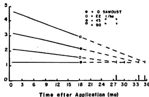
Figure 3.--Effect of rate of application on the decomposition of sawdust in a Florida nursery (after Munson, 1983). Return to ambient level is extrapolated to be 28 mo for 22 t/ha, 34 mo for 45 t/ha and 35 mo for 90 t/ha.
