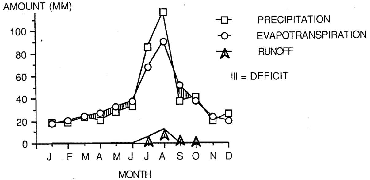
Fig. 2. Observed precipitation and estimated evapotranspiration and runoff for a site near Los Alamos, NM (after Lane and Barnes, 1987).
